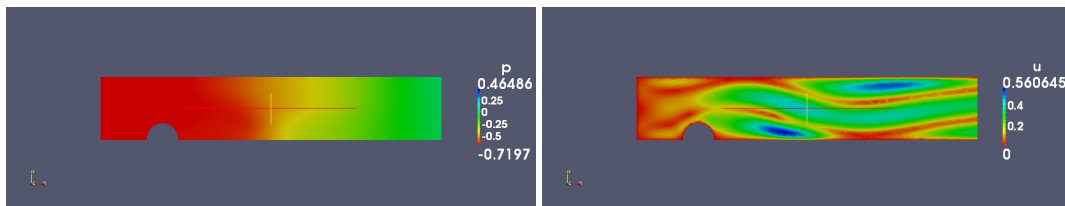
Figure 2: The Numerical pressure p_h and Numerical velocity u_h for Navier-Stokes equations at time t=8
