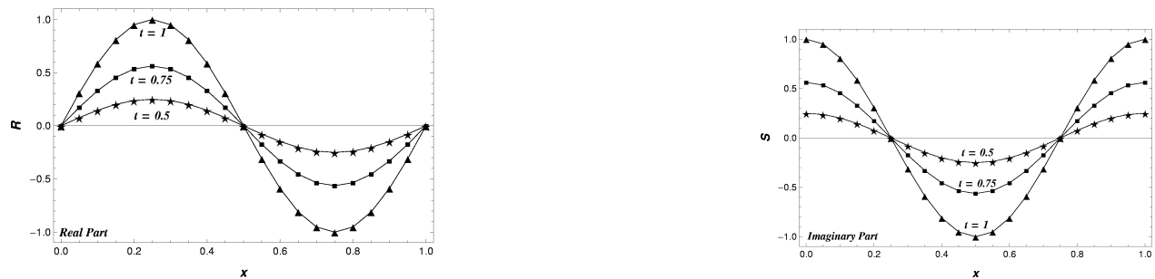
Figure 1: The comparison of the exact(lines) and numerical solutions for \gamma = 0.5 , N = 40 and \Delta t = 0.002 at t = 0.5 (stars), t = 0.75 (squares), and t = 1 (triangles).
